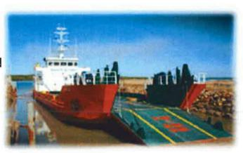
N.T. (Upgrading to BV) Survey current Length Overall 45.50 m L.B.P. 41.172 m Breadth 11.00 m Total Deck Area 290 sqm Depth 3.20 m Draft designed 2.50 m Draft max 2.50 m **GRT** <500 t
